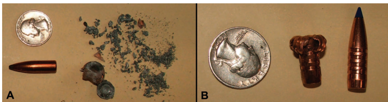
FIGURE 3. The remains of Pb and copper bullets fired into a water barrel from a .30-06 rifle. (A) Unfired Pb core bullet (with a copper alloy jacket) next to remains from a fired bullet of similar type. Tiny bullet fragments provide a great deal of surface area allowing for increased absorption of Pb once ingested by scavengers. (B) Unfired copper bullet next to the remains from a fired bullet of similar type. Photos courtesy of Clinton Epps (C. Epps and D. Sanchez personal communication).
